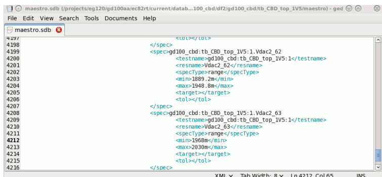
Figure 6.8: maestro.sdb holding the limits for the DAC test shown above
