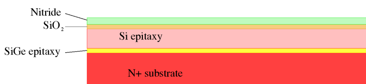
Figure 3.15: Preparation of the wafer
