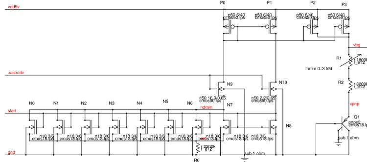
**Fig.1.1:** Example of a simple weak inversion bandgap
