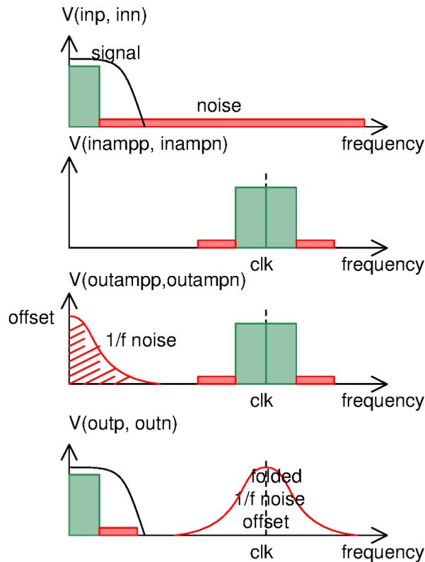
**Fig.2:** Spectral distribution of the signals at different positions of the signal chain
