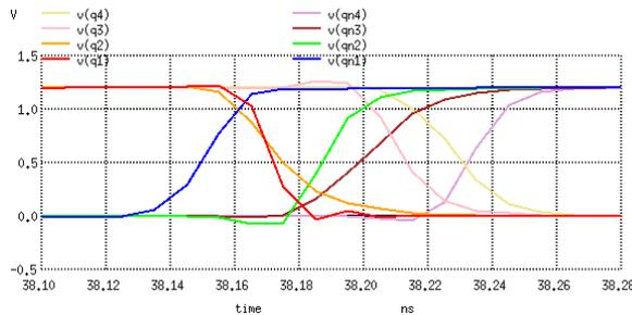
**Fig.4:** Simulation of the synchronizer chain
