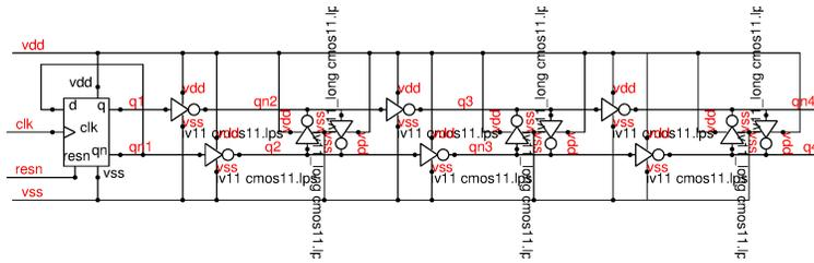
**Fig.3:** Divider with successive synchronizer latches
