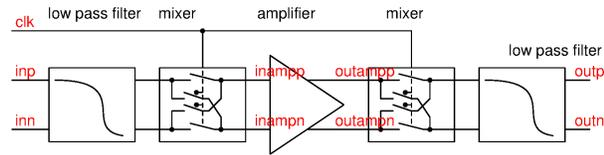
**Fig.1:** Concept of a chopper amplifier
